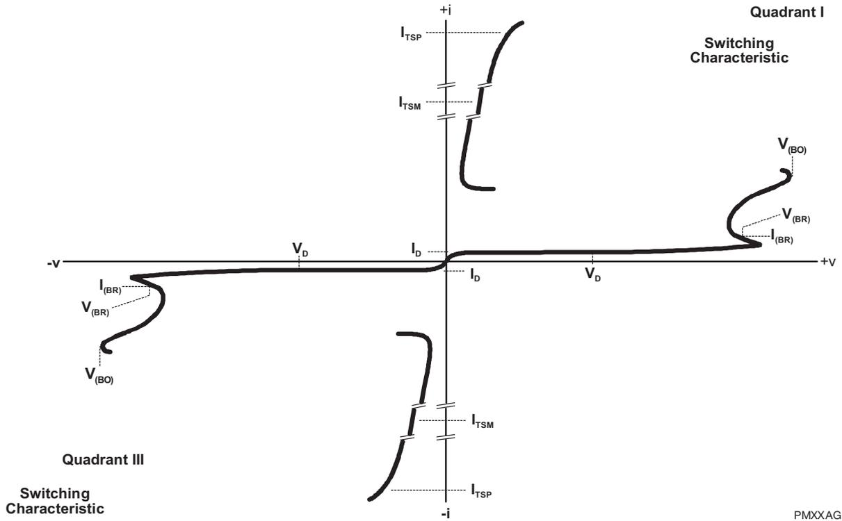
**Figure 1. Voltage-Current Characteristic for the T and R Terminals**
