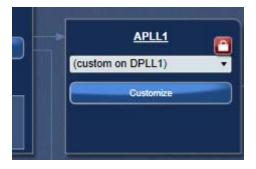
Click on the "Customize" button and ignore the initial Timing Commander error. Enter the values as shown in Figure 11 below to get a VCO of 614.4MHz.
