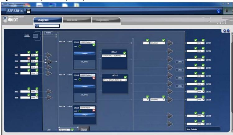
To associate an input clock with a sync signal (such as 1PPS, for e)xample, to associate a sync signal IN1 (1PPS) to IN02 (10MHz)), click on the Input Buffer of IN02 (the triangle symbol following frequency entry box), a sub-configuration window for IN02 is shown below. In the window, IN01 is selected as sync signal.
