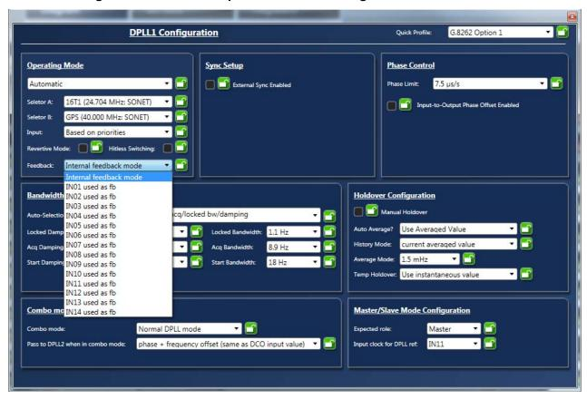
In "Bandwidth and Damping" section, there are two options to select DPLL's bandwidth and damping factors during start, acquisition and locked phases:
