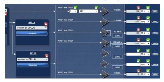
Finally, FRSYNC & MRFRSYNC can be configured, if needed. Change FRSYNC & MFRSYNC to 1PPS. By default, the duty cycle of sync outputs is 50/50. If a pulse is desired, click on the applicable check box. The pulse width is based on OUT01 clock period.
