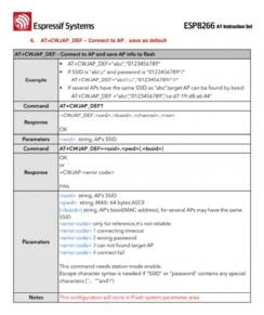
Example page from the AT command set guide – this one demonstrates how to connect to a WiFi access point.
