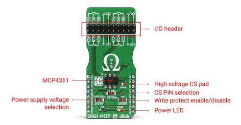
DIGI POT 5 click has one 2x10 pin standard, 2.54mm pitch header used to connect the four potentiometer terminals. There are three SMD jumpers onboard:
