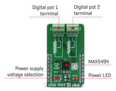
All the communication with the control logic of the MAX5494 is done through the SPI, so all the SPI signals are routed to the appropriate mikroBUS<sup>TM</sup> pins. The CS pin is held high, preventing the SPI communication, so as always - to initialize the SPI communication, the CS pin needs to be pulled LOW by the MCU.
