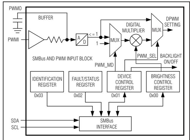
Figure 5. MAX17061 PWM and SMBus Interface Circuit
