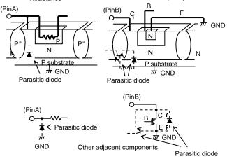
図-1 Simplified structure of a Bipolar IC
