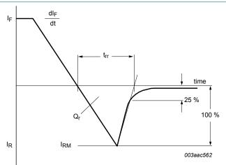
Fig. 12. Reverse recovery definition; ramp recovery
