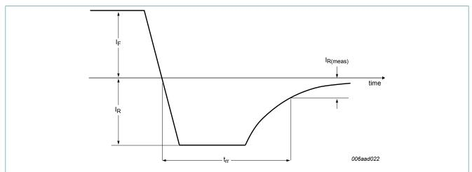
Fig. 11. Reverse recovery definition; step recovery
