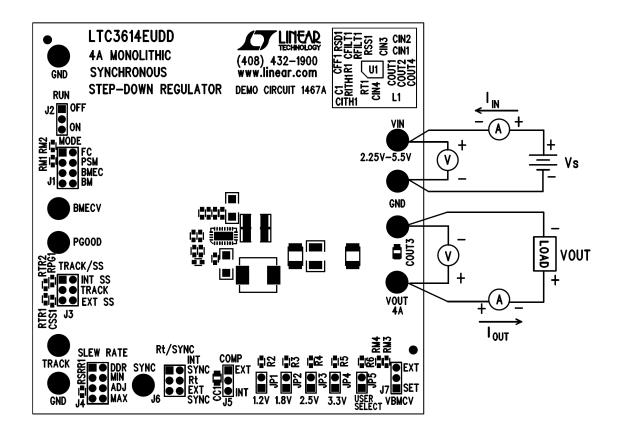
Figure 1. Proper Measurement Equipment Set-Up
