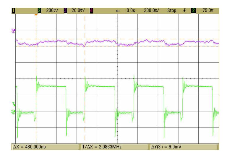
Figure 3. Switch Node & Output Ripple Voltage Waveforms  $V_{\text{IN}}$  = 3.3V,  $V_{\text{OUT}}$  = 1.8V,  $I_{\text{OUT}}$  = 4A
