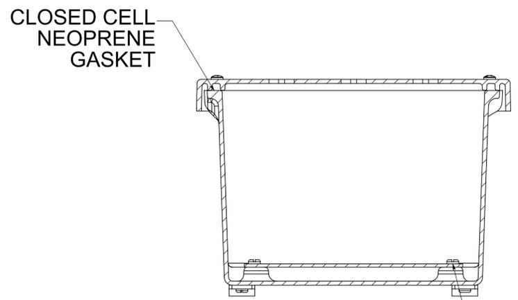
(4) EACH #10-32 BRASS INSERTS AND PLATED CARBON STEEL SCREWS
