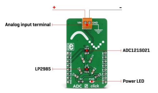
ADC converters in general, use a range of different mechanisms to convert the voltage on their input terminals. The ADC121S021 AD converter uses the SAR, or the successive approximation method for the conversion, which consists of comparing the input voltage with a series of internally generated voltage values. At each step in this process, the approximation is stored in a successive approximation register. The comparing steps are continued until the desired resolution is reached.
