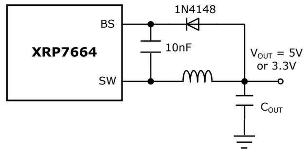
Fig. 17: Optional External Bootstrap Diode where V<sub>OUT</sub> = 5V or 3.3V
