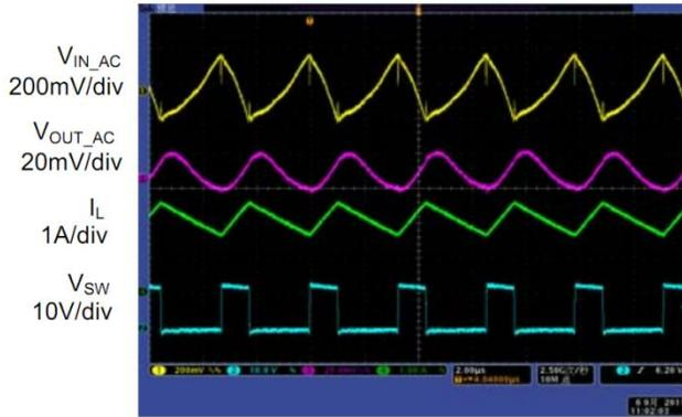
Fig. 10: Output voltage ripple,  $I_{OUT}=2A$
