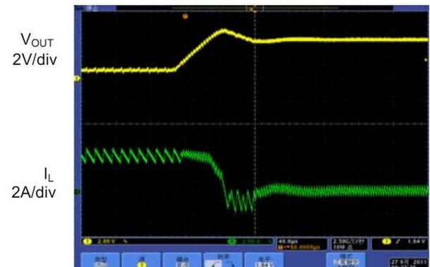
Fig. 15: Short-circuit recovery,  $I_{OUT}=2A$
