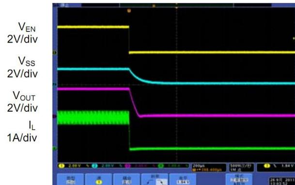
Fig. 13: Enable turn off ( $R_{LOAD}=1.6\Omega$ )
