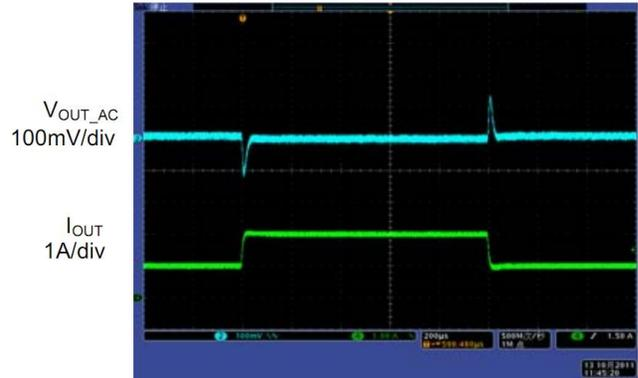
Fig. 11: Load transient ( $I_{OUT}=1A$  to  $2A$ )
