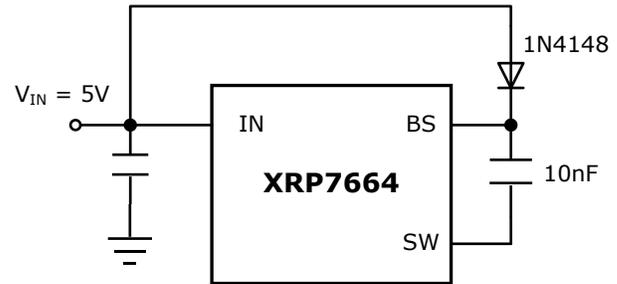
Fig. 16: Optional External Bootstrap Diode V<sub>IN</sub>=5V Fixed
