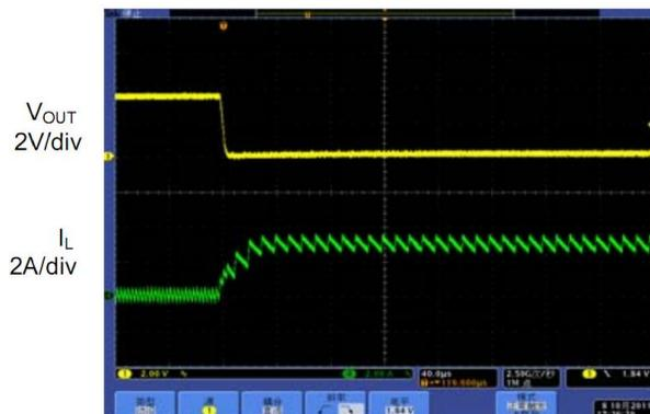
Fig. 14: Short-circuit protection,  $I_{OUT}=2A$
