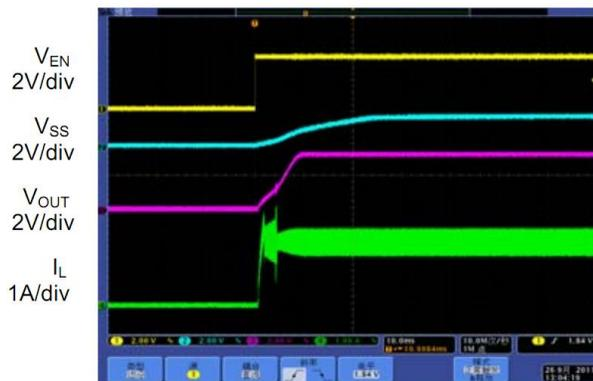
Fig. 12: Enable turn on ( $R_{LOAD}=1.65\Omega$ )
