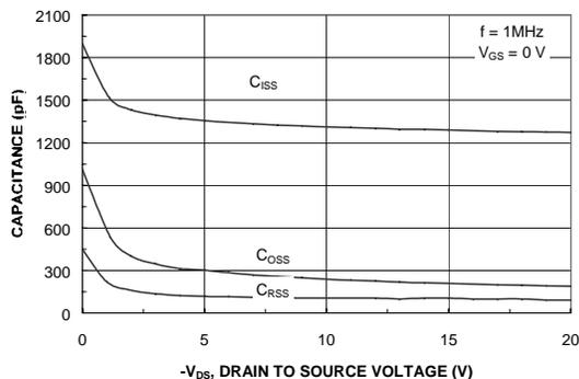
Figure 8. Capacitance Characteristics.
