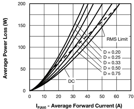
Fig. 6 - Forward Power Losses Characteristics (Per Leg)
