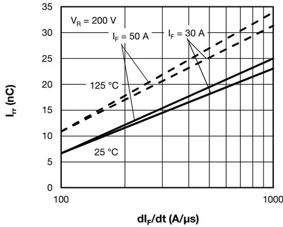
Fig. 9 - Typical Reverse Recovery Current vs.  $di_F/dt$
