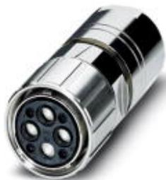
Cable connector, straight, Screw locking, M58, number of positions: 4+3+PE, type of contact: Socket, Crimp connection, shielded: yes, cable diameter range: 17 mm ... 25 mm
