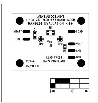
Figure 2. MAX9634 EV Kit Component Placement Guide— Component Side
