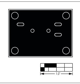
Figure 4. MAX9634 EV Kit PCB Layout—Solder Side
