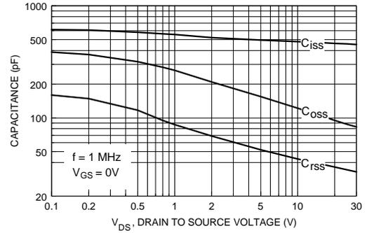
Figure 8. Capacitance Characteristics.
