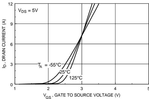
Figure 5. Transfer Characteristics.
