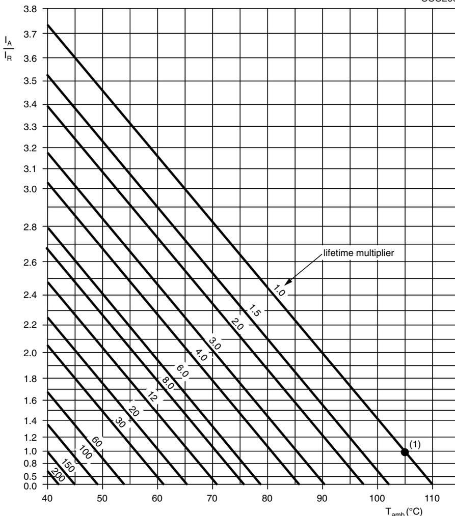
$I_A$  = actual ripple current at 100 Hz or 120 Hz
