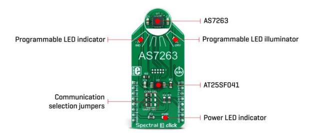
The measurements from the photo elements are digitized by the 16bit ADC converter and processed by the Spectral\_ID engine. Besides the raw values of the six color elements, the engine calculates all the calibrated values available on this device and outputs them as
