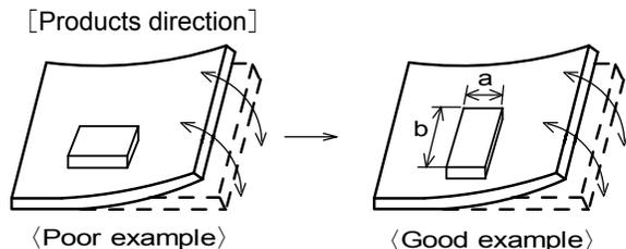
Products shall be located in the sideways direction (Length:  $a \cdot b$ ) to the mechanical stress.
