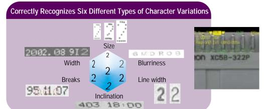
Printed characters such as expiration dates, lot numbers and date codes can vary in shape, size and line width based on the printing method and conditions. The QUEST algorithm ensures that the six most common types of variations are always recognized correctly.
