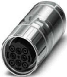
Cable connector, straight long, Screw locking, M40, Number of positions: 2+3+PE, Type of contact: Socket, Crimp connection, Shielded: Yes, Cable cross section: 9 mm...14 mm
