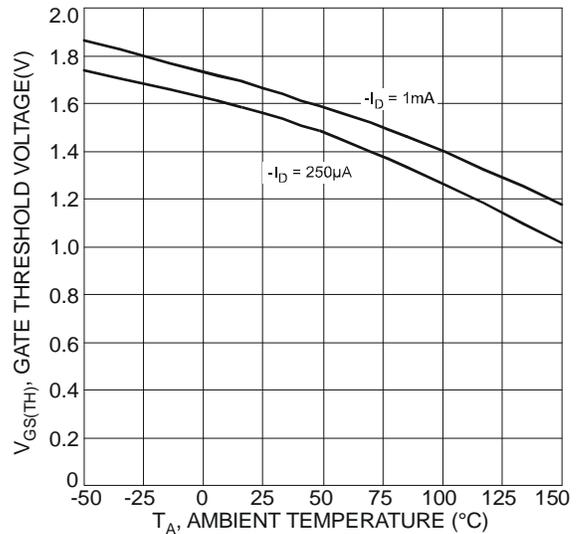
Fig. 8 Gate Threshold Variation vs. Ambient Temperature
