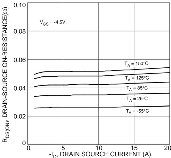
Fig. 5 Typical On-Resistance vs. Drain Current and Temperature
