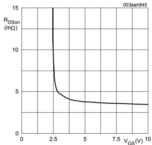
$T_j = 25\text{ }^\circ\text{C}; I_D = 25\text{ A}$
