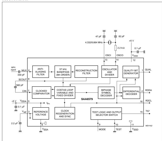
Via pin MODE two different crystal frequencies can be used.
