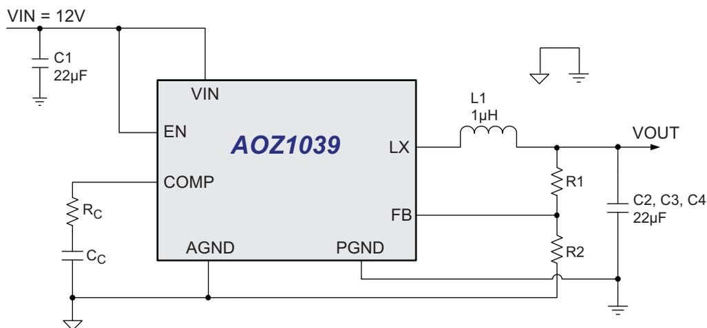
Figure 1. 1.05 V 8 A Synchronous Buck Regulator,  $F_s = 450$  kHz
