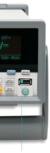
USB port for flash memory devices (8846A) provides convenient data storage and transport
