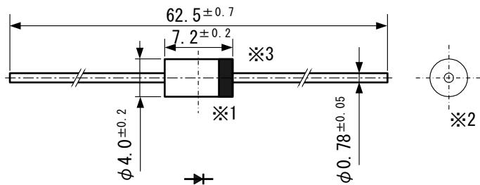
\*1 The allowance position of Body against the center of whole lead wire is 0.5mm(max.)
