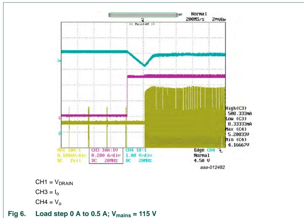
In the worst case (see [Figure 6](#)), the output voltage drops to 4.17 V which fulfills the USB-charger specification 1.1.
