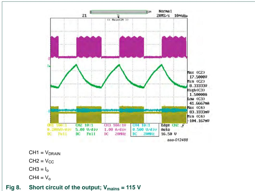
At 230 V, the average output current during a short circuit is 610 mA. The input power is 0.44 W.
