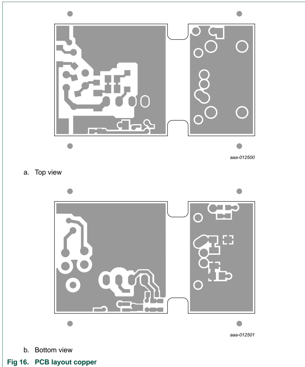
**Fig 16. PCB layout copper**
