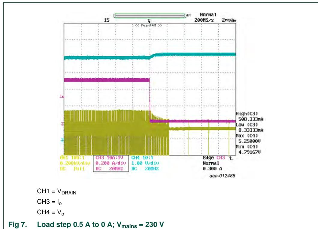
After the load step from 0.5 A to 0 A, the output voltage rises from 4.8 V to 5.25 V.
