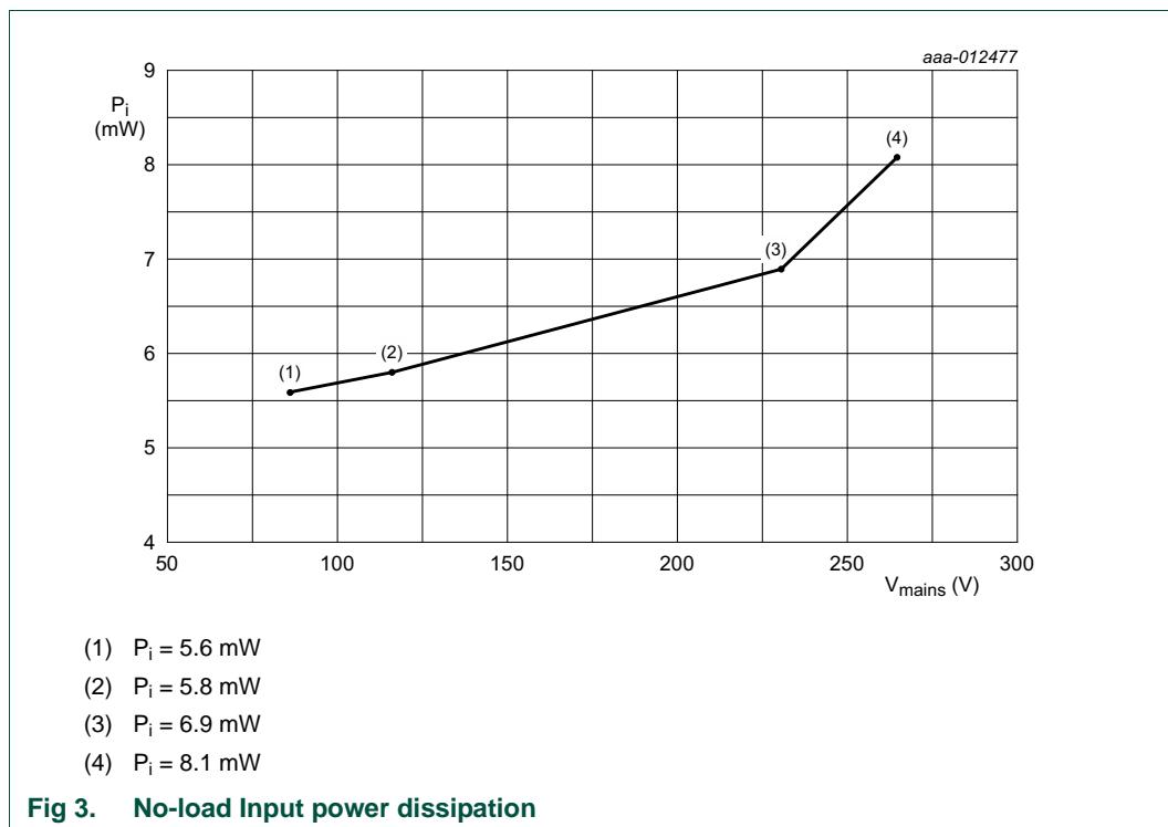
**Fig 3.** No-load Input power dissipation
