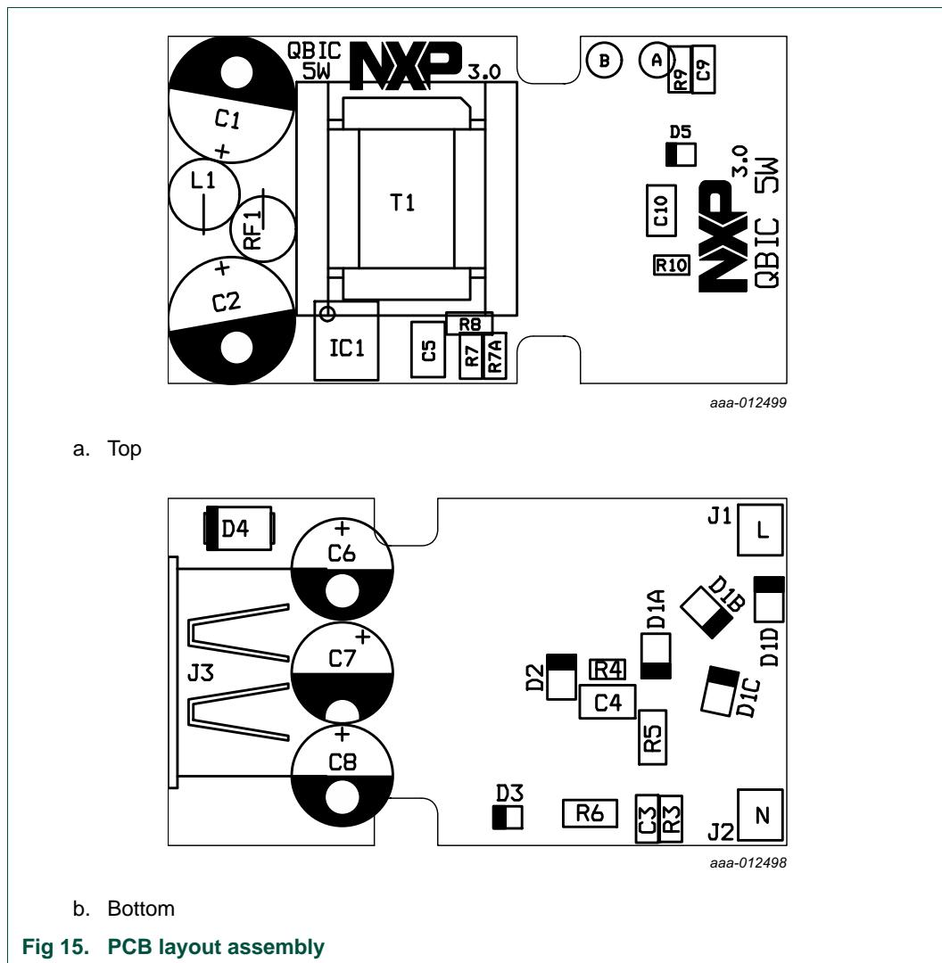
**Fig 15. PCB layout assembly**
