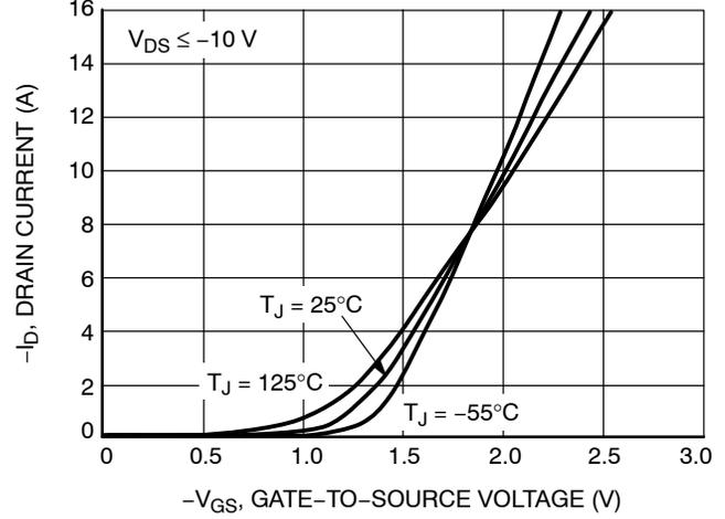
Figure 2. Transfer Characteristics
