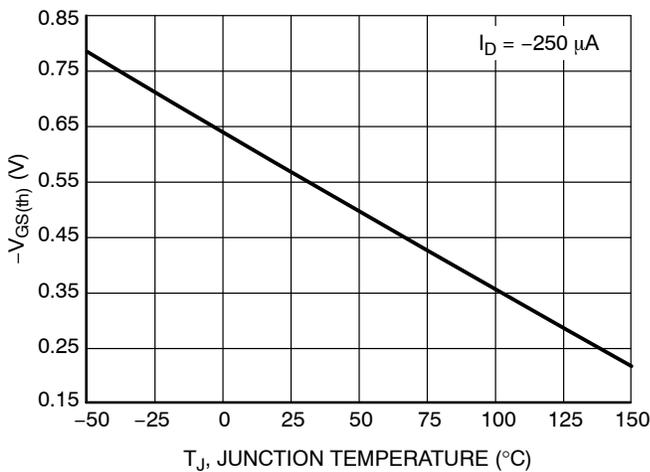
Figure 11. Threshold Voltage
