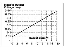
Fig. 6-2 Output voltage vs. output current in normal mode at 24V input, typ.
