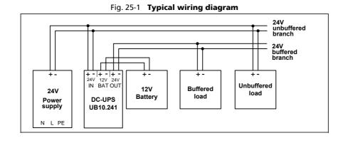
(4) Install the fuse when the wiring is finished.
