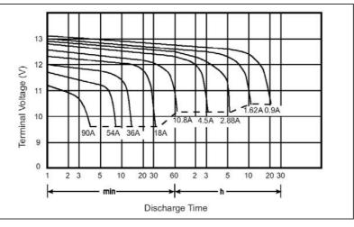
Fig. 9-2 Typical discharging curve of a typical 17Ah battery, curve taken from a manufacturer's datasheet
