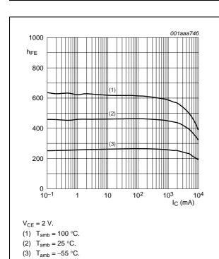
Fig.6 DC current gain as a function of collector current; typical values.
