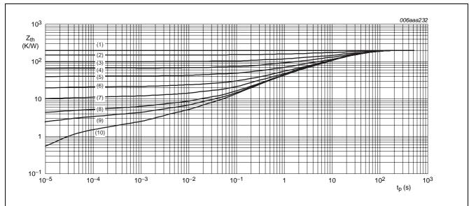
Mounted on FR4 printed-circuit board; standard footprint.
