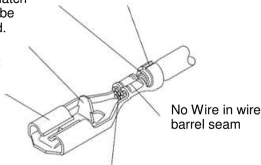
No Wire in wire barrel seam
